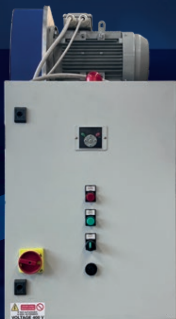
QUADRO CON INVERTER CONTROL PANEL WITH INVERTER
